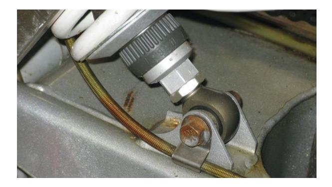
"Offset can also be incorporated into the front axle mount."
