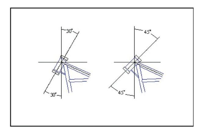
Rake is the rearward inclination of the steering head as measured through the center of the steering stem.
