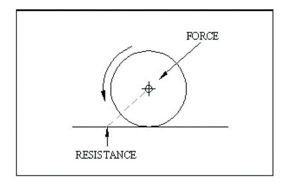
Inclining the fork rearward and therefore applying the force at an angle induces stability.
