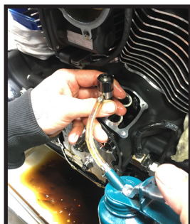
Manually pump up lifters
