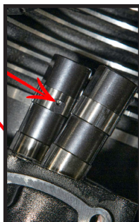
Install lifter oil feed holes facing each other
