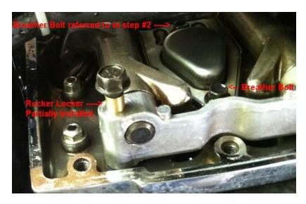
Pull a bolt out of the right side of the plate, (facing forward on the bike) this is the side that locks the shaft. Insert the Rocker Locker in the hole; they are tapered, put the small end in the hole.
