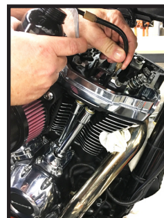
Manually pump up pushrods & rocker arms
