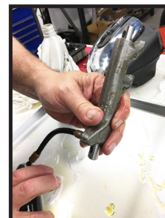
Manually pump up pushrods & rocker arms
