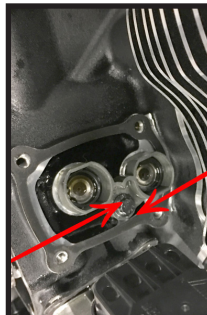
Install lifter oil feed holes facing each other
