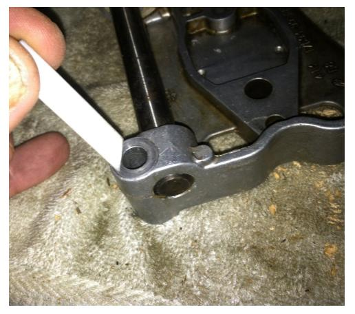
Using the Teflon Centering Tool to line up the notch in the Rocker Shaft
