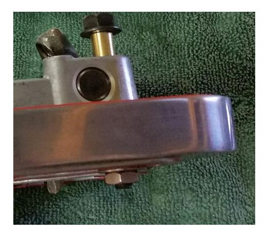
This photo shows the Rocker Locker being pressed into the Rocker Cover Inner by slowly turning the bolt with a wrench, while holding the nut stationary with another wrench.
