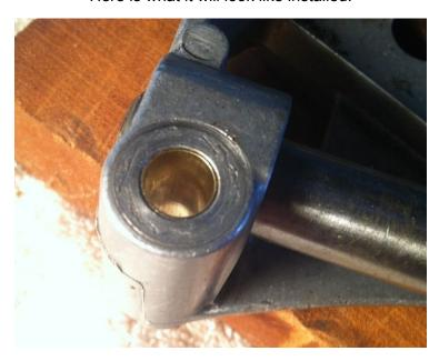
**3B**. *Bike Installation:* For installation on the bike, you do not have to remove the plate, but it needs to be loose so that the Rocker Lockers can center the plate when it is tightened, it also takes the pressure off the shaft so that is can turn/get the notch lined up, and let the Rocker Locker pull past.
